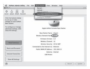
3.If your network is password protected, you should choose Equivalent Network Password from the Base Station menu as shown above. Write down the value that appears in the dialog as shown below. This is your network password.
